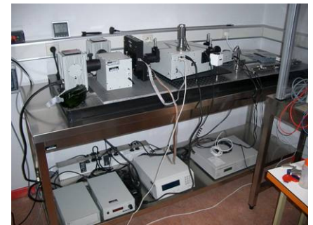
Figure 66 : Optical bench at Demelab (with Deuterium & Tungsten lamps, chopper, monochromator, integrating sphere, \Theta -x-y-z translation stage,...).
