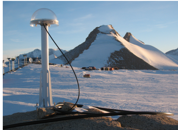
Figure 24: GPS antenna installed at the Princess Elisabeth base in Antarctica
